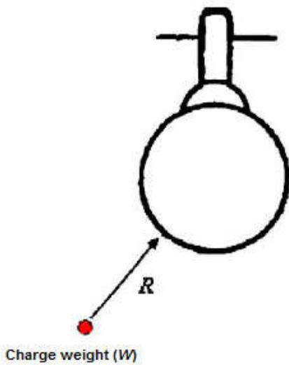
Fig.2. Hull shock factor
