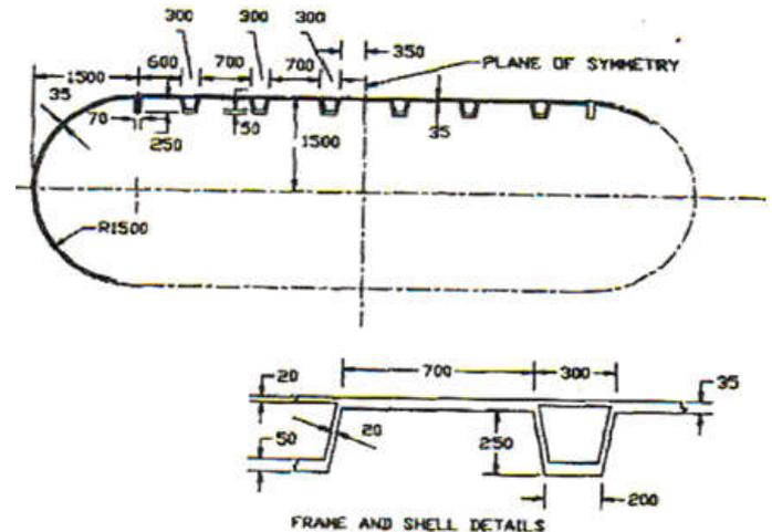
Fig. 3. Physical model of submersible hull
