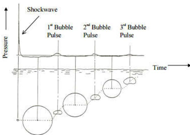
Fig.1. Pressure waves and bubble phenomena of underwater explosion
