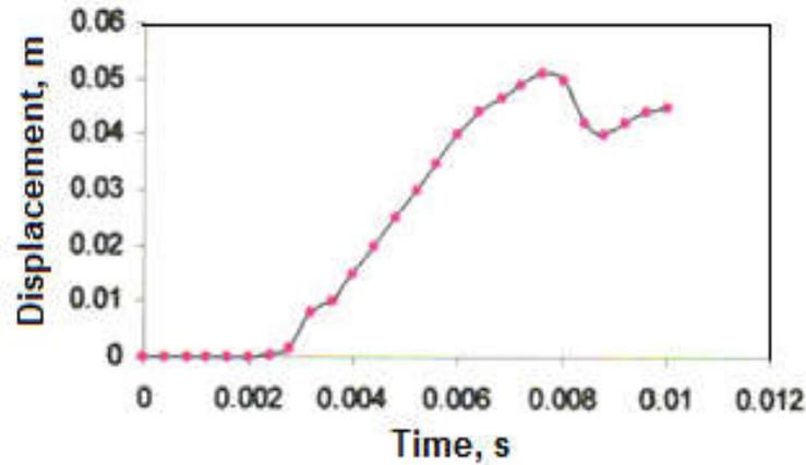
Fig. 5. Displacement-time history for charge weight of 25 kg
