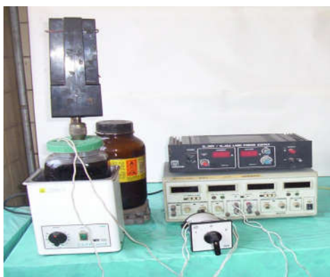
Photograph 1. Electrolytic oxidation system
