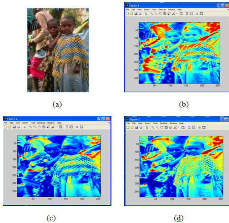
Figure 4.2. (a) Original RGB image (b) extracted Red components, (c) extracted Green components, (d) extracted Blue components
