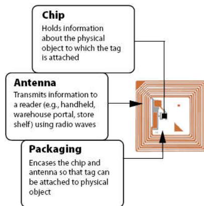
Fig. 1. Showing the elements of RFID system
