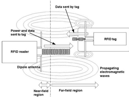
Fig. 3. Showing the schematic of far-field coupling between a reader and a tag [9]
