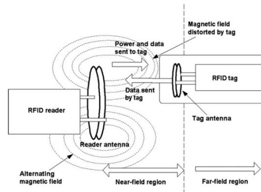
Fig. 2. Showing the schematic of near-field coupling between a reader and a tag [9].
