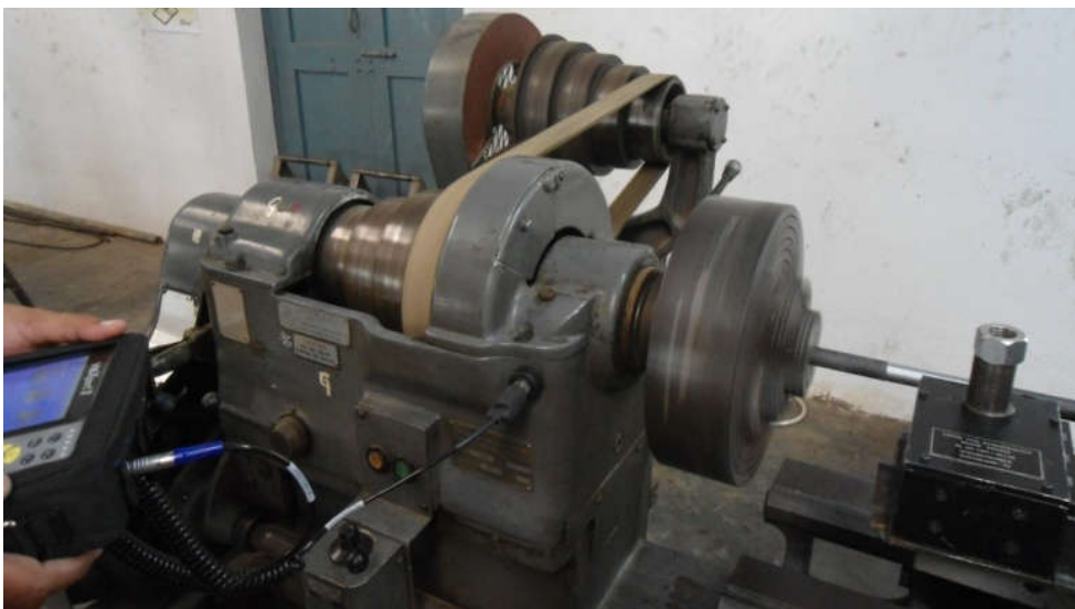
Figure 2.4. Experimental setup for spindle vibration level measurement in horizontal direction (Z)
