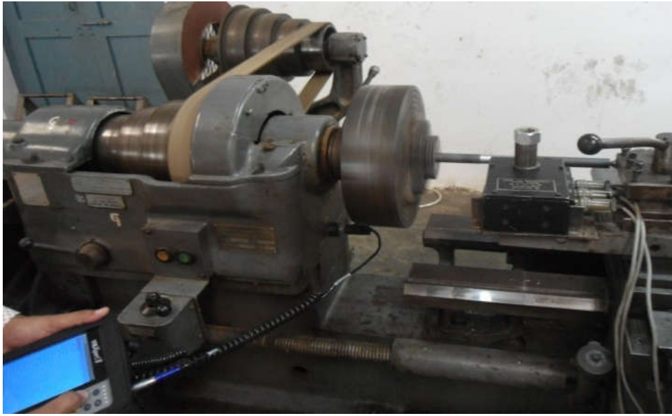
Figure 2.2. Experimental setup for spindle vibration level measurement in axial direction (X)
