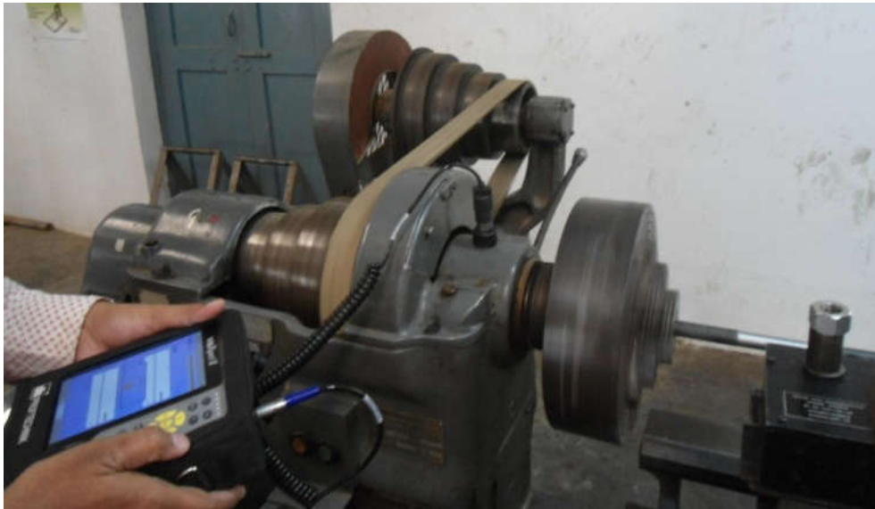
Figure 2.3. Experimental setup for spindle vibration level measurement in vertical direction (Y)
