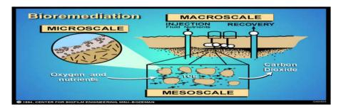
Fig. 13: In-situ bioremediation. Source: Stewart (2008)
