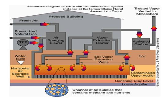
Fig. 11. Air-Sparging. Source: Stewart (2008)
