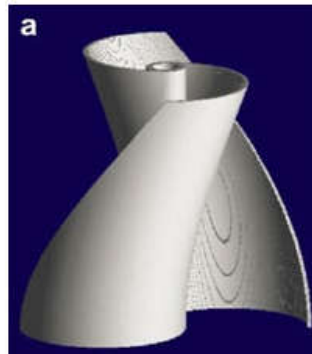
Figure (21) M.A kamojo Helical Savonius Rotor [10] with twisted angle 90^\circ
