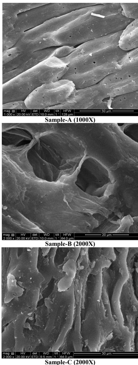
**Figure 10. SEM image of fracture surface of different sized Arecanut husk samples in Alkaline hydrolysis Pretreatment**
