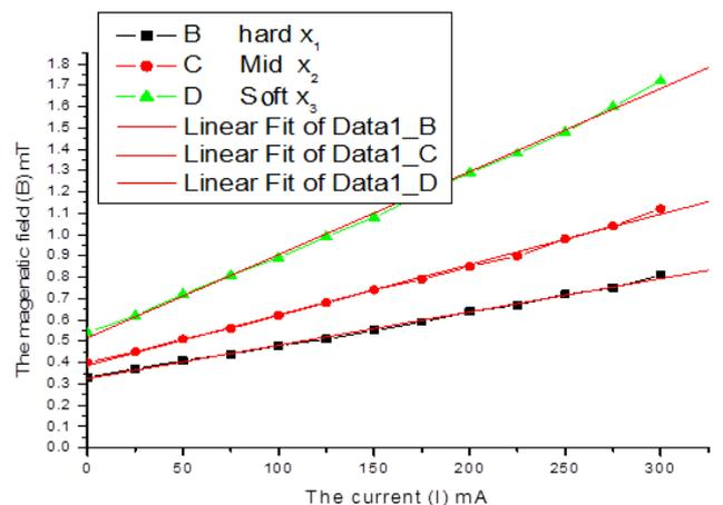
Figure 2. The relation between magnetic flux B and Current I for different size Iron Fillings
