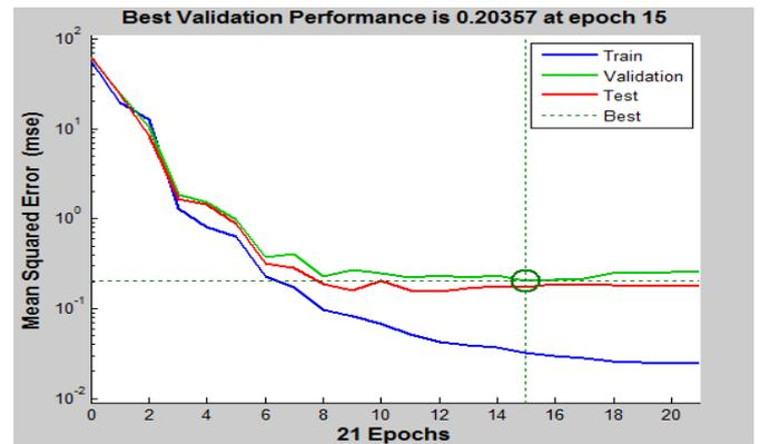
Figure 2. Neural network training performance of solar radiation for all the eighteen locations
