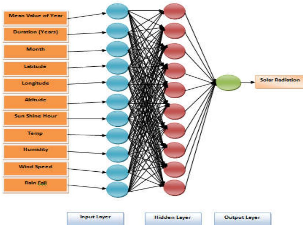
Figure 1. ANN architecture used for prediction in this present work
