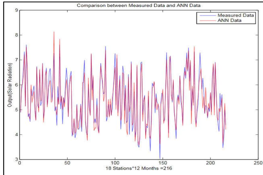
**Figure 4. Comparison of measured and estimated solar radiation data**
