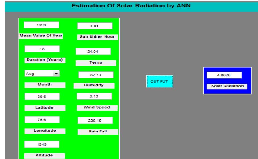
**Figure 5. Graphical user interface for the estimation of solar radiation**
