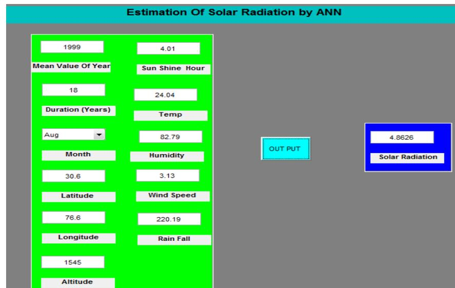
**Figure 5. Graphical user interface for the estimation of solar radiation**
