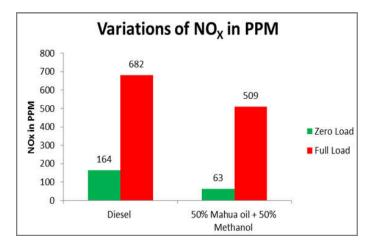
Fig. 5. The variations of Nitrogen dioxide for Diesel and Mahua oil blended with Methanol at Zero Load and Full Load
