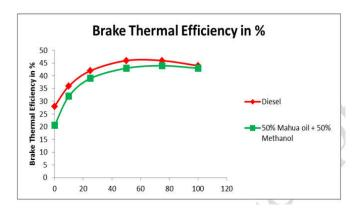
Fig. 3. The variations of Brake Thermal Efficiency for Diesel and Mahua oil blended with Methanol at different Loads
