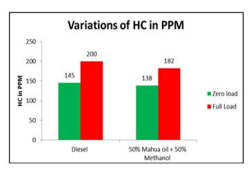
Fig. 4. The variations of Unburnt Hydro Carbon for Diesel and Mahua oil blended with Methanol at Zero Load and Full Load
