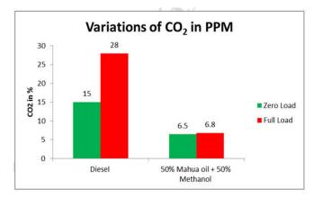
Fig. 6. The variations of Carbon dioxide for Diesel and Mahua oil blended with Methanol at Zero Load and Full Load
