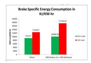
Fig. 2. The variations of Brake Specific Energy Consumption for Diesel and Mahua oil blended with Methanol at Zero Load and Full Load
