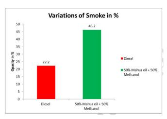
Fig. 7. The variations of Smoke for Diesel and Mahua oil blended with Methanol at Zero Load and Full Load
