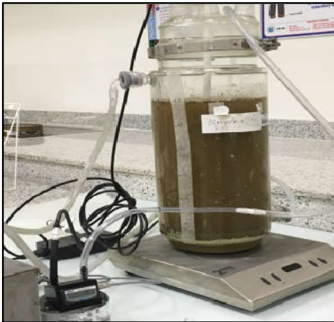
Fig. 2. Step two in preparing the inoculum: Set the bio-reactor to be ready receiving the 6 l solution of Horse Dung Slurry
