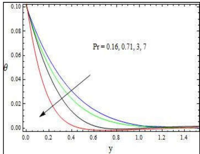
Fig. 12. The Temperature Profile for  $\theta$  against  $Pr$  with  $R=2; t=0.1$
