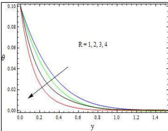
Fig. 11. The Temperature Profile for  $\theta$  against  $R$  with  $P=0.71; t=0.1$
