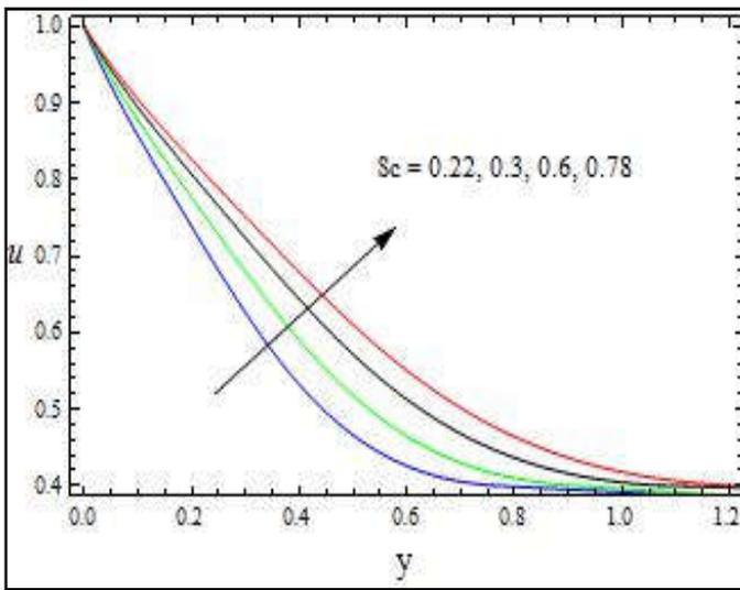
Fig. 10. The velocity Profile for  $u$  against  $Sc$  with  $\alpha = 1; M=2; D=1; P=0.71, R=1; t=0.1; Gr=5; Gm=10$
