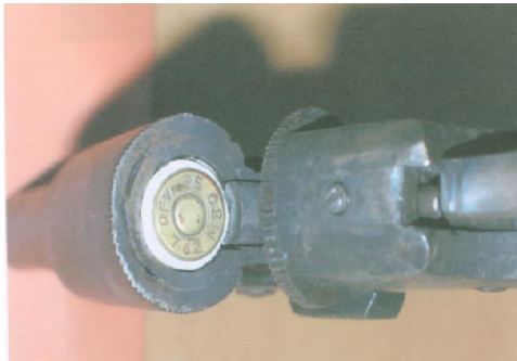
Figure 2. 7.62mm rifle cartridge with cotton thread packing
