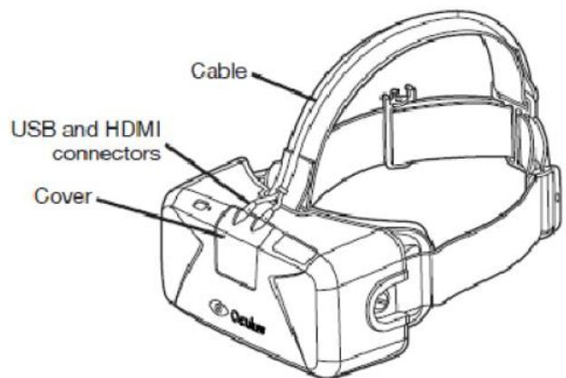
3. Connect the head set cable to the computer CPU: The head set cable has two connectors one is HDMI and the other is USB. Plug both the connectors to the computer.
