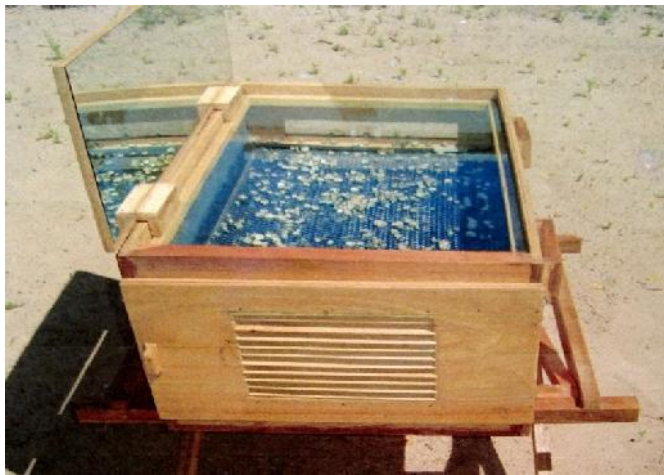
Figure 1. Assembled Solar cabinet dryer showing contents on drying racks with reflector to boost solar collector, with a louvered like vented door
