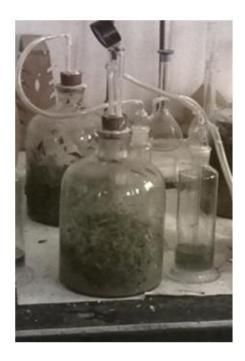
Figure 1. Single Biomethantion unit (Digester)
