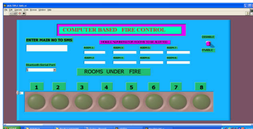
Fig. 4. Front panel for the designed firefighting system
