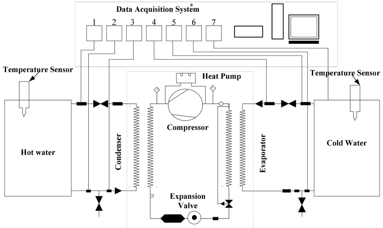
Fig. 4. Heat pump monitoring system
