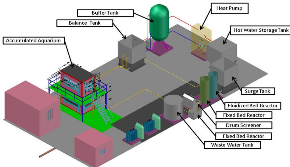
**Fig. 3. Schematic diagram of vertical aquarium plant for energy management**
