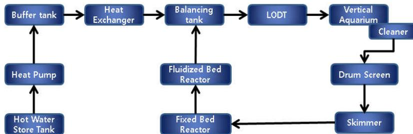
**Fig 2. Application targeted heat pump layout**
