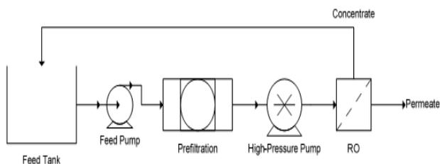
**Fig. 2. Schematic diagram of an RO desalination unit**
