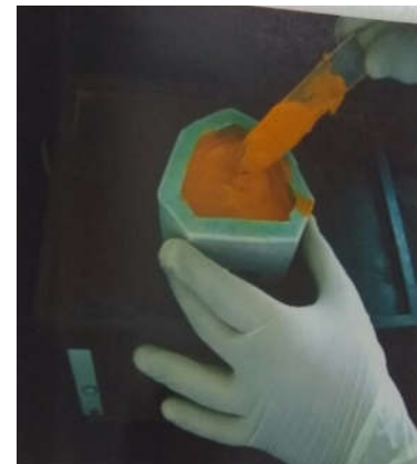
Fig 6 Pouring of silicone rubber mould
