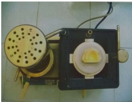
Fig 7. Vaccum adaptation of bioacrylic sheet
