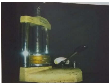
Fig 10. Flask under Hydarulic pressure
