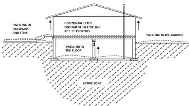
Figure 2. Ground movement associated to the construction of a shallow foundation over an expansive soil (Fredlund and Rahardjo, 1993)
