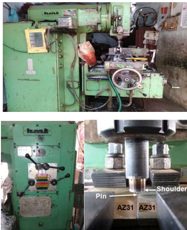
Fig. 2. FSW on vertical milling machine
