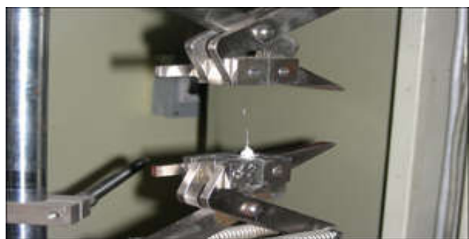
Figure 3. Tensile bond strength testing on Zwick Universal Testing Machine
