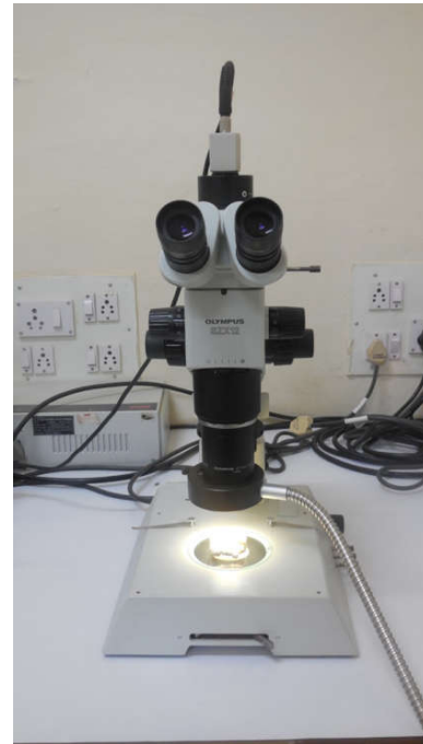
Figure 3. Optical stereomicroscope (Olympus, SZX 12, Japan), 3 Chip CCD Camera (Proview, Media Cybernetics, USA) with image Pro-Plus Software (Version 4.1.0.0)
