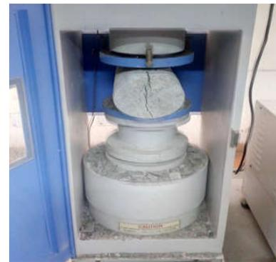
Fig.9. Concrete cylinder with crack
