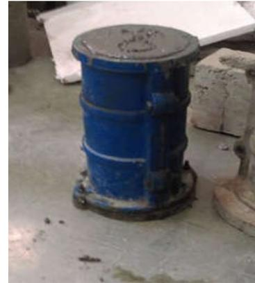
Fig.8. Cylinder mould
