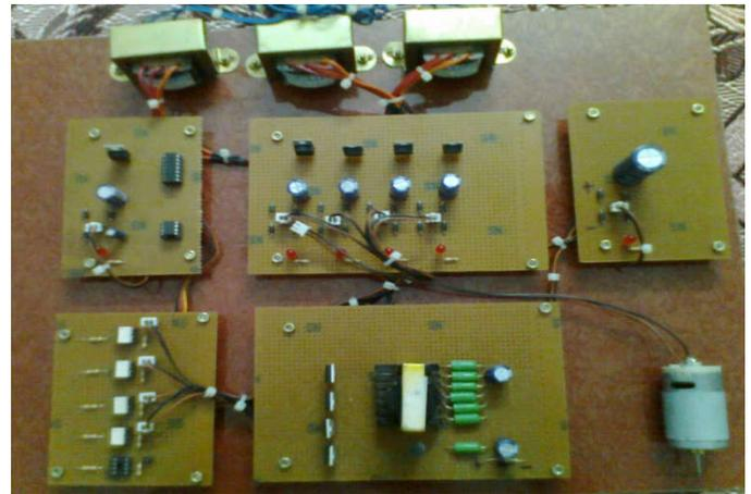
Fig. 11. Prototype of Interleaved Coupled Inductor Boost Converter
