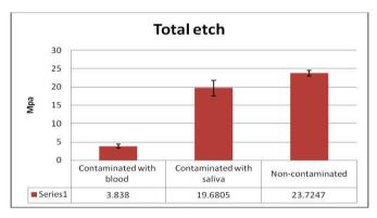
Figure 2. Mean (±SD) compressive strength for total etch group
