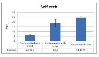
Figure 1. Mean (±SD) compressive strength for self etch group
