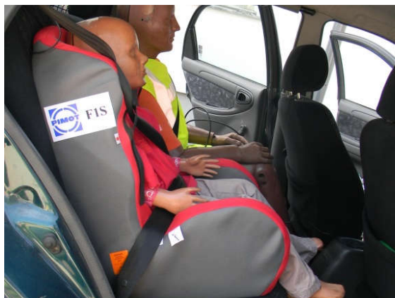
Fig. 3. One of the FS seats with the CHILD dummy, installed in the test car
