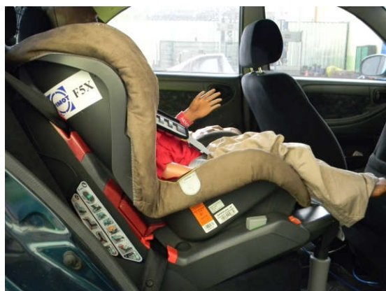
Fig. 4. One of the FX seats with the CHILD dummy, installed in the test car
