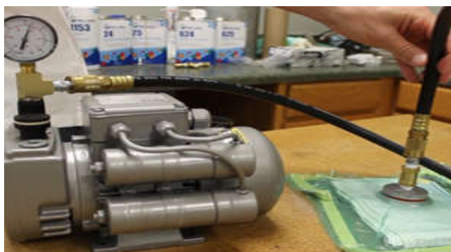
Figure 3. Vacuum bagging technique
