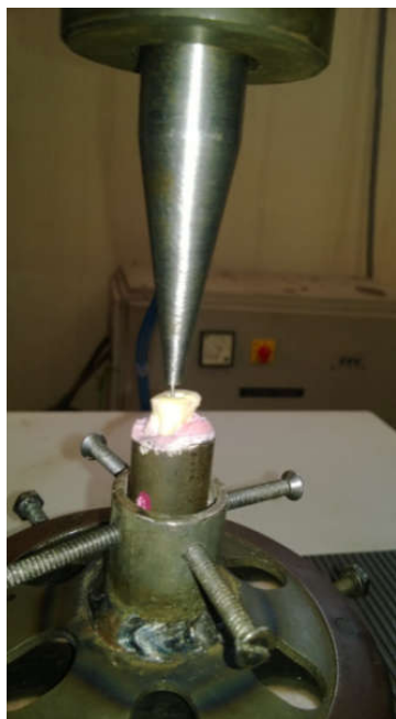
Figure 3. A sample being tested with 1mm thick cylindrical stylus under Universal Testing Machine
