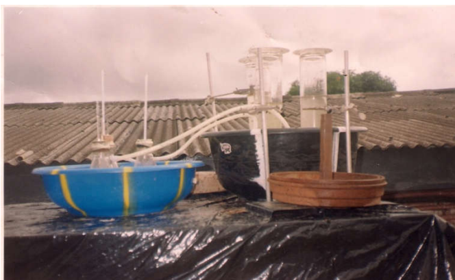
Fig. 1: Digester set-up for biogas production of the wastes.
