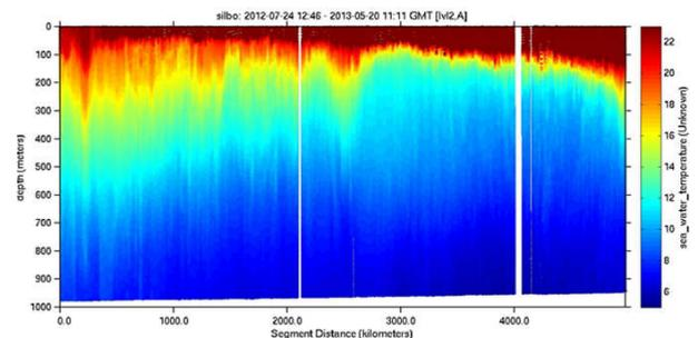
**Figure 3. Course of the Silbo glider (left) and vertical temperature profile measured by the glider (right)**
