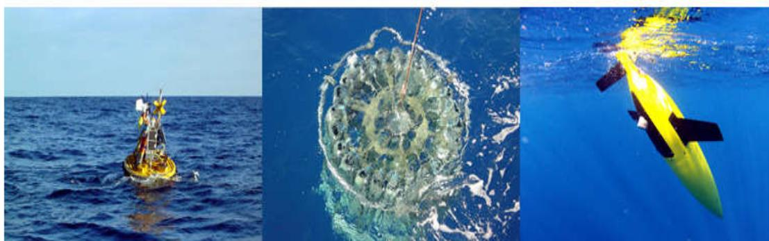
**Figure 2. A weather-oceanographic Dolan buoy (left), water sampling rosette (centre), autonomous underwater vehicle glider (right)****Table 2. Total number and type of buoys installed in each area of Macaronesia within R3M**
