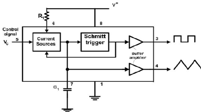
Fig.(1) A block diagram of 566 IC.
