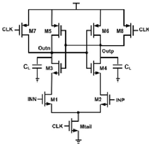
Schematic diagram of the conventional dynamic comparator.
