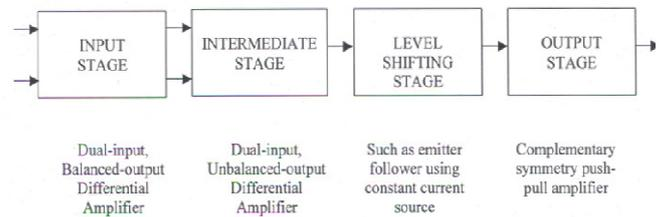
Fig. Block diagram of Op-Amp
