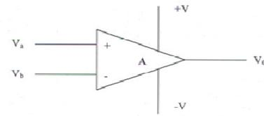
Fig. Op-amp schematic diagram
