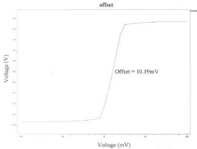
Fig. 5.1.1 Transfer function with offset of folded-cascode OTA
