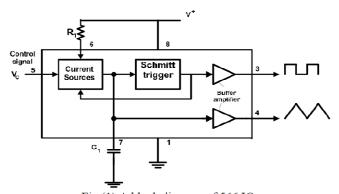
Fig.(1) A block diagram of 566 IC.
