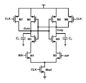
Schematic diagram of the conventional dynamic comparator.
