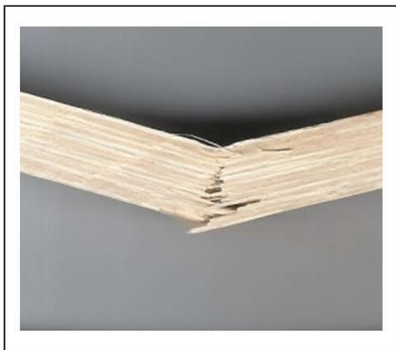
Figure 10. The pattern of failure of static bending test for the three species of date palm midribs (splintering tension)
