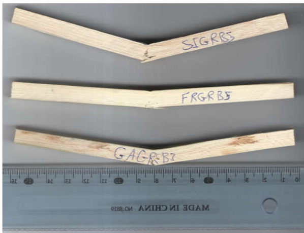
Figure 9. Comparison between the bending Young's modulus for three species of date palm midribs
