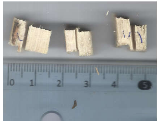
Figure 15. Comparison between the transverse shear strength for three species of date palms
