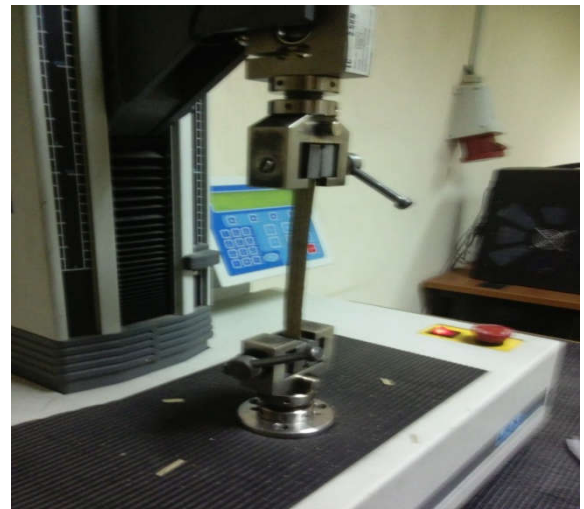
Figure 7. The tensile test sample for date palm leaflets while performing tensile test
