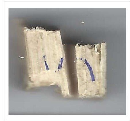
Figure 16. The pattern of failure of shear test for the three species of date palm midribs in longitudinal direction (splintering and shearing)
