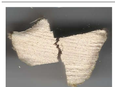
Figure 17. The pattern of failure of shear test for the three species of date palm midribs in transverse direction ( splintering and shearing)
