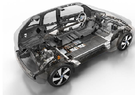
Figure 3. All body panels of BMW i3 made of carbon fiber reinforced plastics (18). SOURCE: BMW i3: Cheap, mass-produced carbon fiber cars finally come of age, By Bill Howard on July 30, 2013 at 1:40 pm. https://www.extremetech.com/extreme/162582-bmw-i3-will-bmws-new-ev-finally-be-the-breakthrough-for-carbon-fiber-cars
