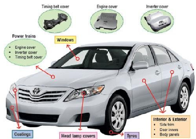
Figure 4. An illustration of the use of nanocomposites in automobile components. Source: Polymer nanocomposites drive opportunities in the automotive sector. Nanowerk Spotlight, http://www.nanowerk.com/spotlight/spotid=23934.php
