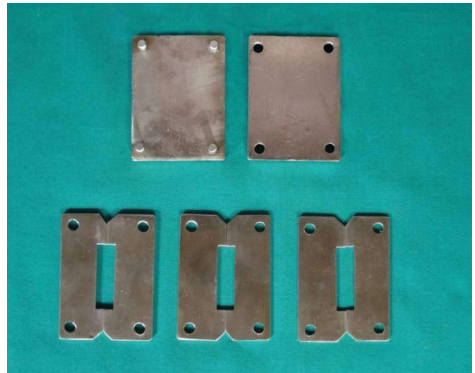
Figure 1. Metal master mold consisting of two metal master plates and three split plates with slots used for fabricating test specimens
