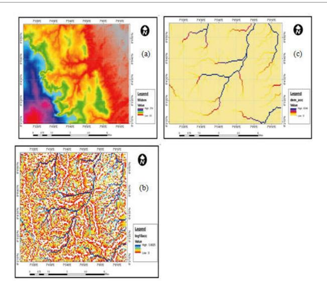
Figure 5. Map showing (a) Digital Elevation Model (b) Flow Accumulation (c) Drainage pattern of Agulu-Nanka and its environs
