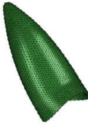
Fig. 3c. Finite element model of the periodontal ligament
