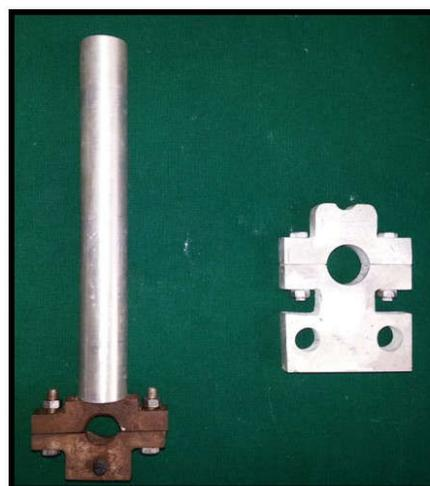
Figure 2. Jig for standardizing tooth preparation
