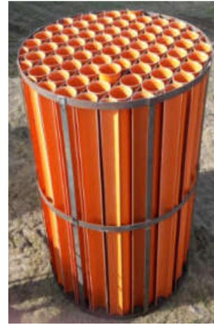
Fig. 5. Adhesive bed - the filling is a "basket" with pipes type A PVC-U S4 UD - roughness after sanding is  $80 \mu\text{m}$
