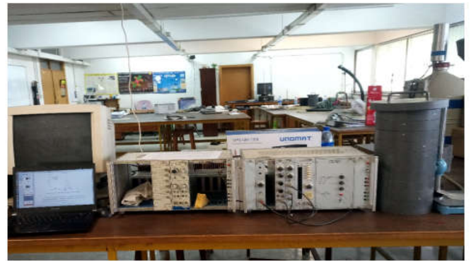
Figure 2. Gamma spectrometry with FJ374 scintillation crystal and Electronic circuits
