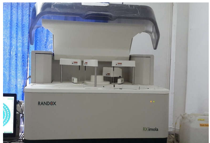
Photograph 1. Randox RX Imola for serum bilirubin analysis using photometric method
