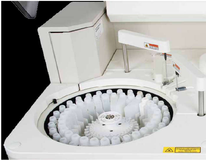
Photograph 2. Randox RX Imola for serum bilirubin analysis using photometric method
