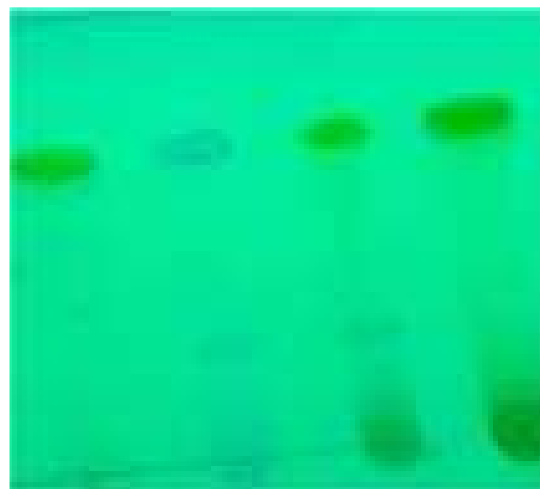
Figure 6. TLC of curcumin (lane 1), cholesterol (lane 2), physical mixture (lane 3), and phytosome 1:1 ratio (lane 4). Solvent system consists of 9.9:0.1 ratio DCM and methanol respectively under UV visible light at 366 nm wavelength.
