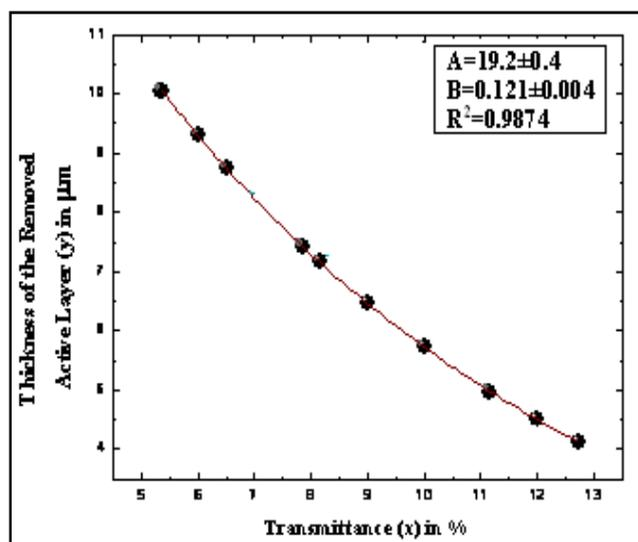
Figure 2. Variation of removed active layer thickness with transmittance
