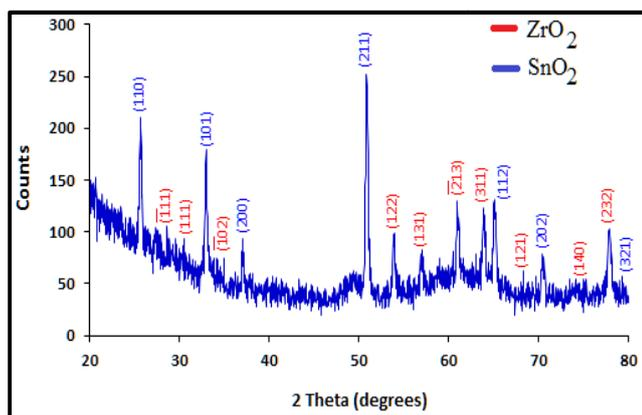
Fig. 1. XRD of  $\text{Zr}_{(0.50)}\text{Sn}_{(0.50)}\text{O}_4$  powder
