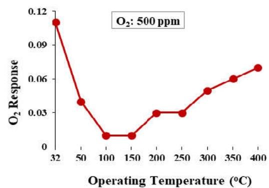
Fig. 6. O<sub>2</sub> response Vs. op. temperature
