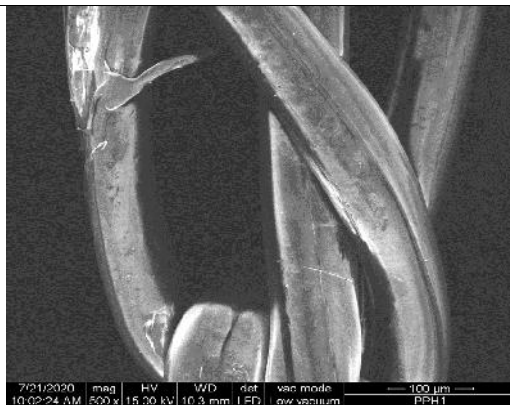
Fig. 4. SEM images of PP yarns after treatment
