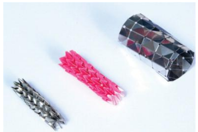
Fig4. Models of an origami stent graft that can be used in the treatment of esophageal cancer. The models are made from stainless steel tubes to obtain good geometrical compatibility during expansion, though in reality much more flexible materials are used.
