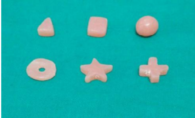
Fig. 1 Different shapes of test specimens In this image six types of shapes made from cold cure acrylic resin was showed
